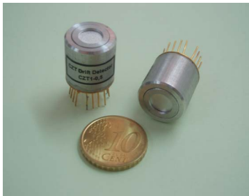
Fig. 2. The CZT detectors mounted in hermetic TO-8 packages. The packages contain also the Peltier coolers, the FET and the PT100 sensors.
