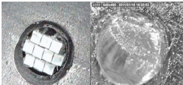
FIGURE 3: (a) The optical coupling scheme and (b) photographs of the Sci-Fi and clear fiber prepared for coupling.
