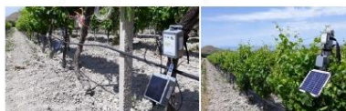
Xylem sap flow rate by a methodology based on T-Max method (TT-Wine, TreeTalker Wine, Nature 4.0 SB srl, IT)
