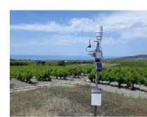
Weather station (Meter environment, ATMOS41)
