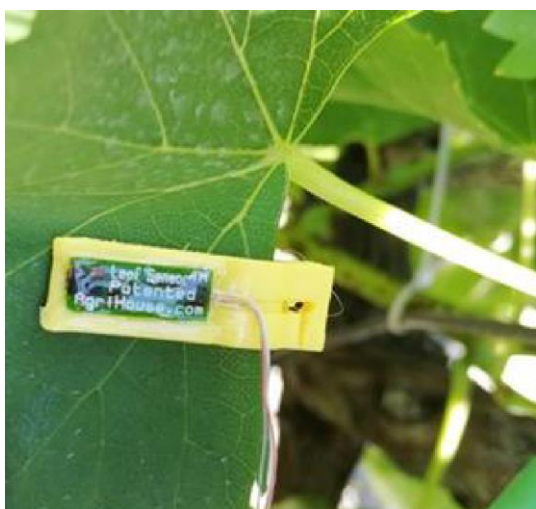
Figure 2.6 Leaf sensor of Agrihouse company measuring the leaf thickness - Romangia - 2019
