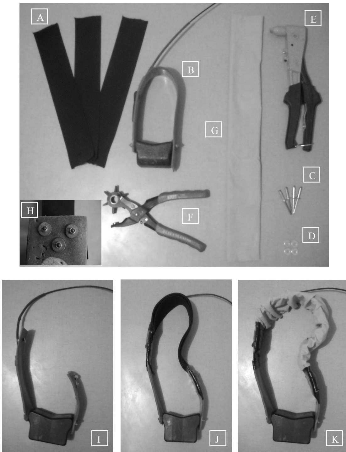
Fig. 1 – Materials deployed to build expandable radiocollars: A) Layers of elastic acrylic tissue. B) Televilt radiocollar TXV-10. C) Pop rivets. D) Spacing washers. E) Riveter. F) Punch pincers. G) leather layer. Assemblage stages: H) Detail of riveted layers on collar. I) Cut collar. J) Collar with acrylic layers assembled. K) Final stage of the device with all parts assembled. See text for major details.
