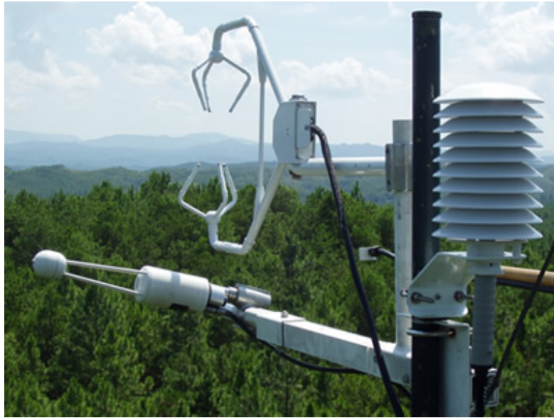
Figure 7. The EC system constituted by a 3-D sonic anemometer an infrared gas analyser, and a temperature and humidity probe.
