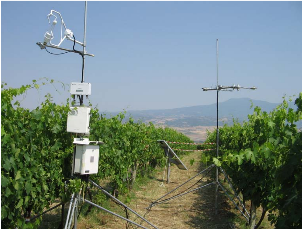
Figure 20. The EC system instrumentation used over grapevine canopy consists of a sonic anemometer, gas analyzer, and net radiometer (Campbell Scientific, Logan, UT, USA)
