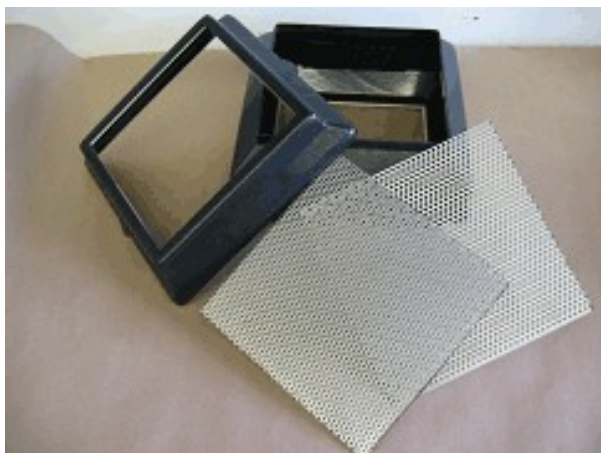
Figure 6. Zeta-box sieving equipment developed by Grant and Cotanch (2005) of the Miner Institute (Chazy NY) in cooperation with Zen-Noh National Federation of Agricultural Co-operative Association of Japan.
