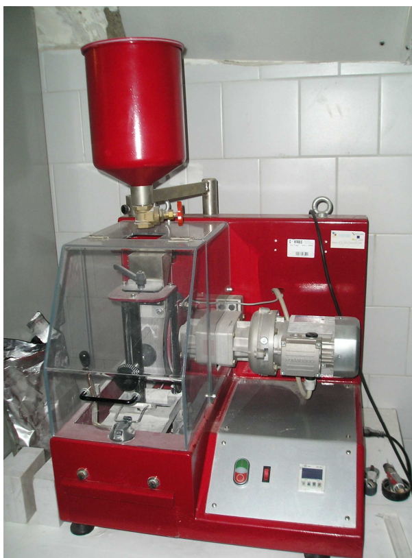
Figura 3.38 – Abrasimetro Controls 48 D 0 471.
