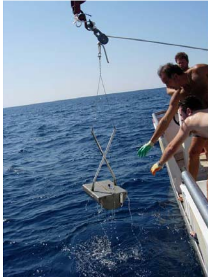
Fig. 2.8. Sampling phase of macrofaunal assemblages with the Van Veen grab.
