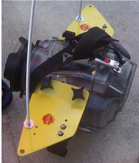
Fig. 4.6. PVC housing for the video recording apparatus employed.
