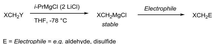
Scheme 2.13: Generation of magnesium carbenoids via magnesium-iodine exchange under non-Barbier conditions.
