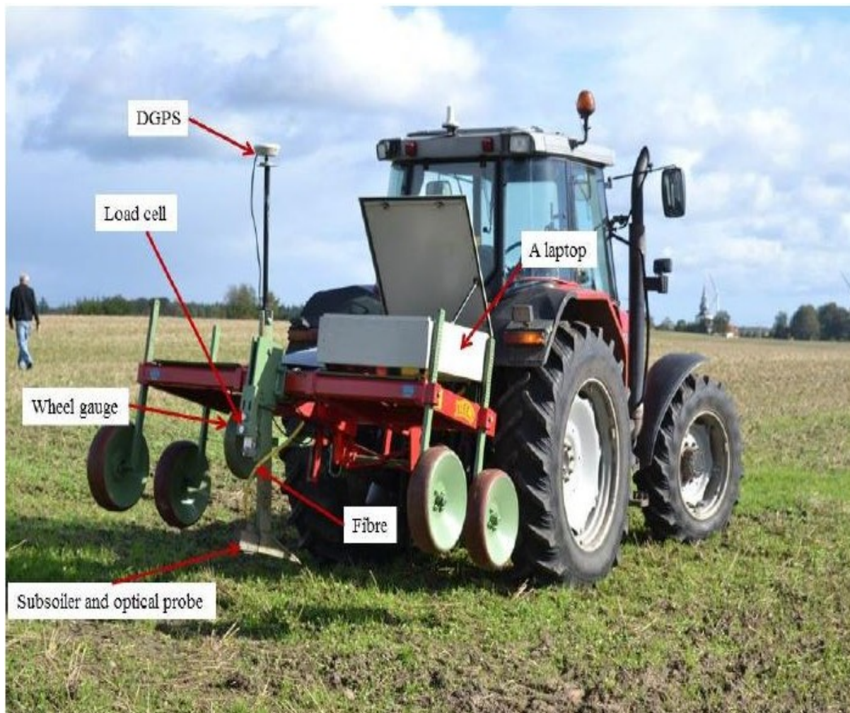
Figure 7. The on-line visible and near infrared (vis-NIR) soil sensor (Mouazen, 2006)
