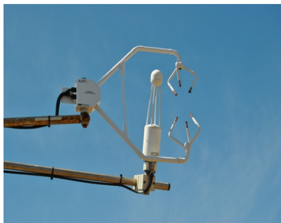
Fig 6.2.2.2. Eddy Covariance instrumentation (sonic anemometer and infrared gas analyzer).
