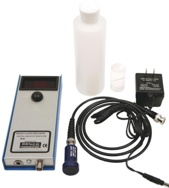
Figure 1: Ultrasound lean meter used to the measurement of dorsal fat thickness
