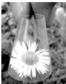
Figure IV.8 High transparency of a resin containing BNC demonstrated by the view on a flower through a corresponding foil.
