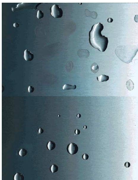
Figure 2.1- Stainless steel substrate coated by spraying of an abrasion resistant, fluorinated hybrid coating (lower part), demonstrating the “easy-to-clean” aspect 18 .
