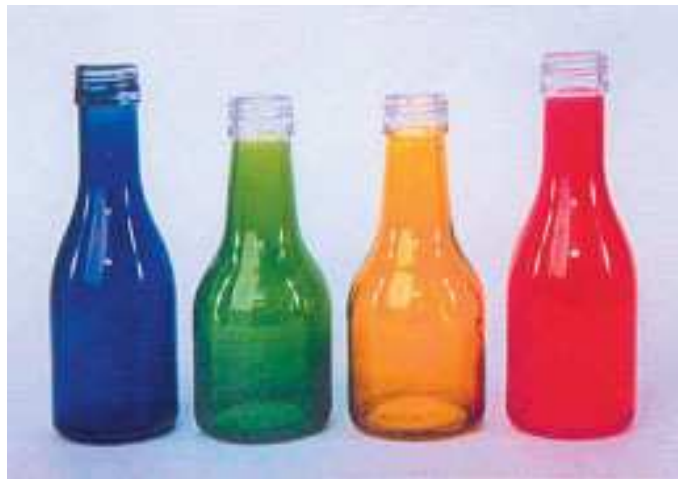
Figure 2.4 -Easy to recycle colored glass bottles coated by hybrid organic-inorganic materials 1 .
