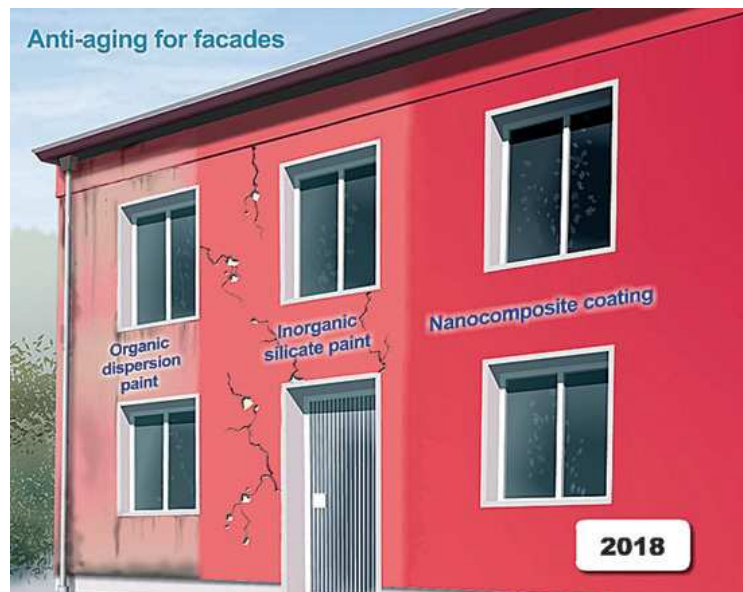
Figure 2.5- The new nanobinder Col.9 combines in one product the different advantages of conventional coating types in terms of low dirt pick-up, chalking and rack resistance, and color retention. (www.col9.com)
