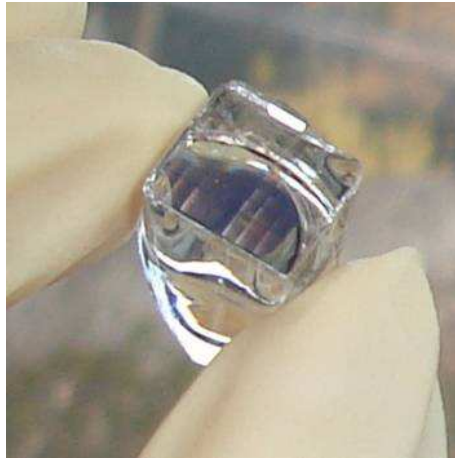
Figure 4.32- Appearance of the PDMS mold after cure at 100°C for 1 h.
