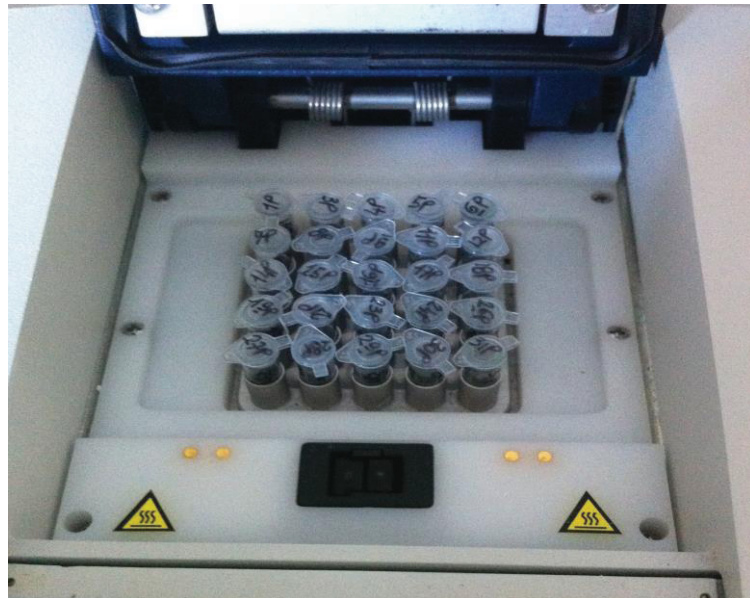
Figure 31. Microtubes with samples for PCR within the plate of thermal cycle.
