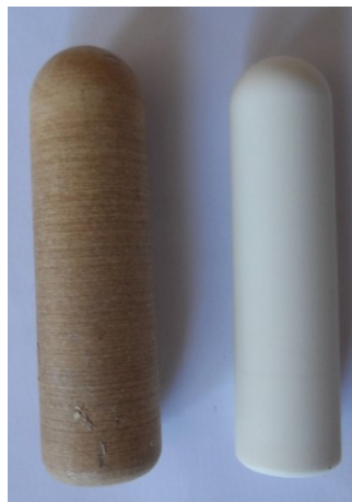
Figure 2.3. Comparison of two ceramic boluses: a) ceramic bolus after permanence in reticulum b) non applied ceramic bolus (control)
