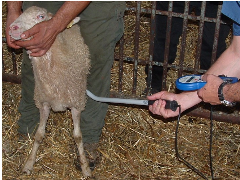
Figure 3. 2. Static reading of electronic bolus in sheep
