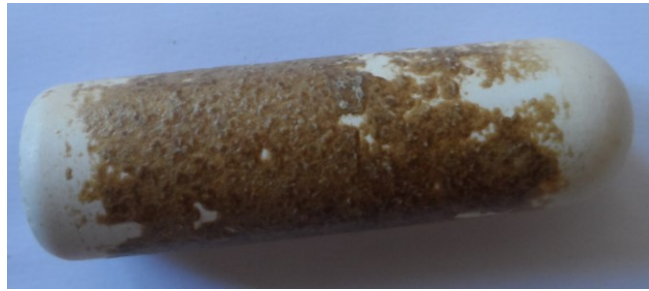
Figure 2.1. Particular of the concretion in a ceramic bolus after permanence in reticulum
