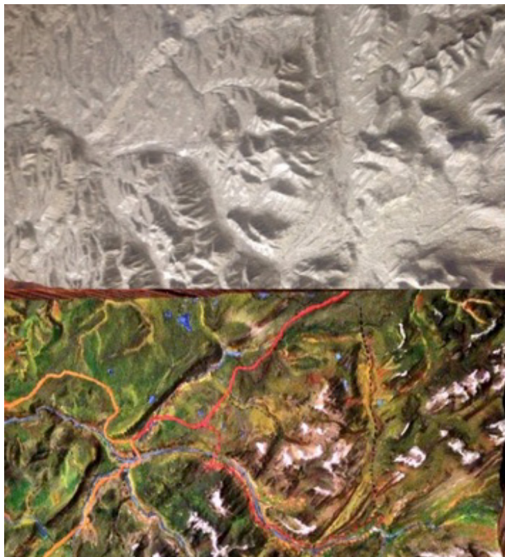
Fig. 32 Example of model printed with 3D printer and then populated/coloured with physical features. Source: http://www.fabbaloo.com/blog/2016/3/30/another-3d-printing-use-case-land-models
