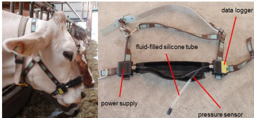
Figure 5. Description of RumiWatch noseband sensor. Adapted from Zehner et al. (2012)
