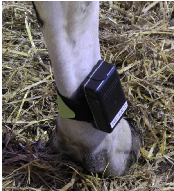
Figure 2. Pedometer fastened on a cow's leg. Adapted from Kajava et al. (2014)
