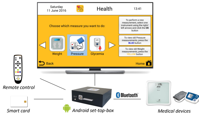
Fig. 2. The HEREiAM TV-based telecare system with the main screen of the Health app.
