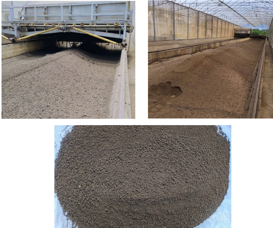
Fig. 61, 62 and 63. Daily turning of sewage sludge for stabilization purposes; end of the channel with stabilized material; stabilized and sieved sludge ready for use in treatments.
