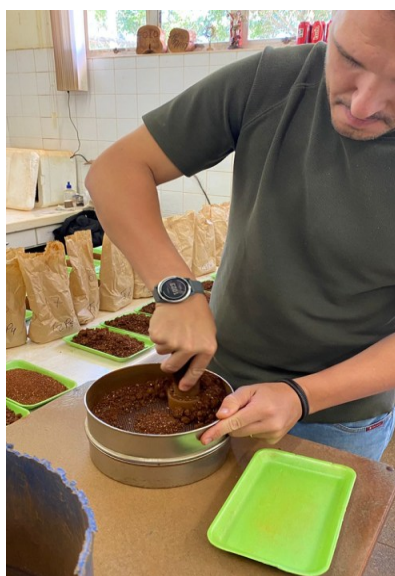
Fig. 78 and 79. Sieving of dry samples and samples ready to be sent for chemical analysis.
