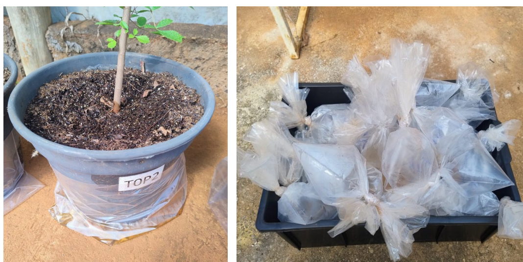
Fig. 84. Leachate collection for pH and electrical conductivity (EC) measurement
