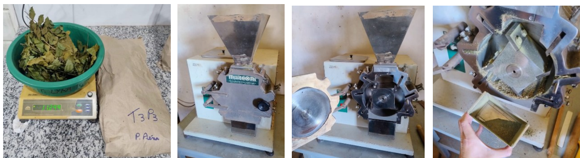
Fig. 100, 101, 102 and 103. Weighing of the dry aerial part (left); grinder used to grind the aerial part (other photos).
