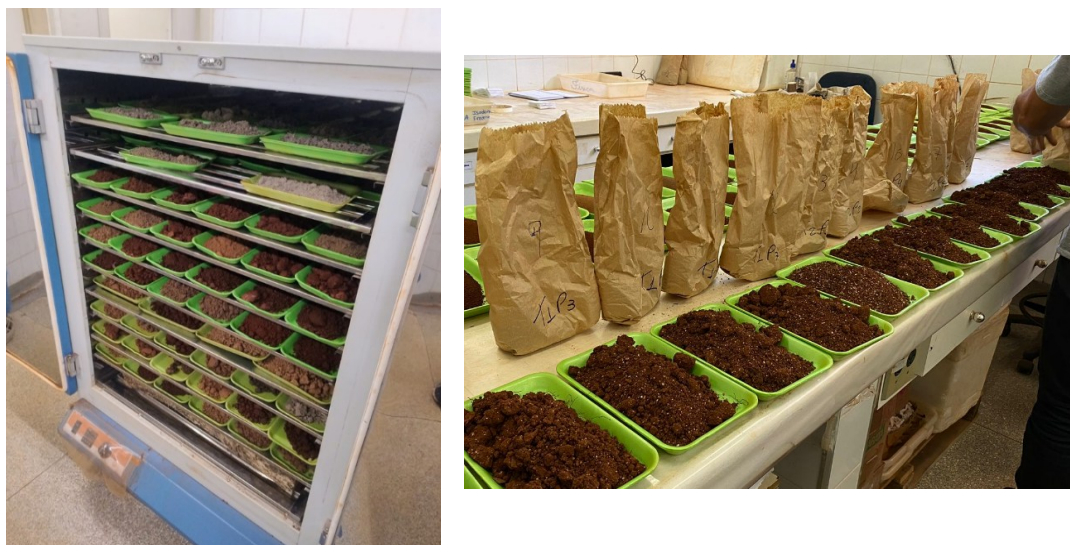
Fig. 76 and 77. Samples inside the forced-air drying oven and then on the bench for further sieving.
