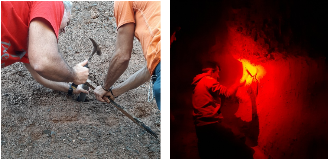
Figure 77. Collecting loose sediment for IRSL dating using a PVC tube during both day and night.
