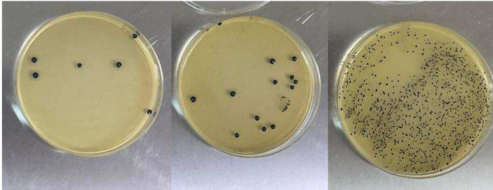
Figure 8.7 S. aureus colonies formed after storing the culurgiones samples in P- PVC for 3, 6 and 24 h
