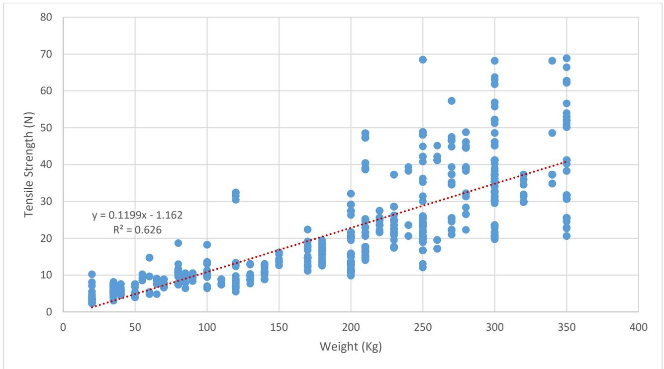
**Figure 16:** graph showing the correlation between weight and tensile strength; the linear equation  $y = 0.12x - 1.16$  is the expression of the model allowing the prediction of tensile strength according to weight with significant accuracy ( $p < 0.05$ )
