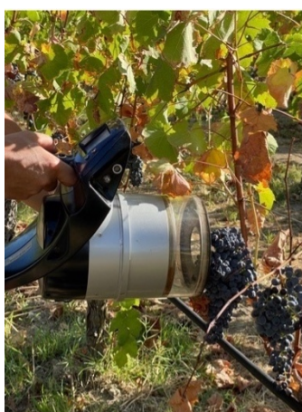
Figure 2. The Multiplex instrument used in the surveys. The fluorescence detectors are placed in the internal area of the instrument, and the interaction with the samples is allowed by the central opening.
