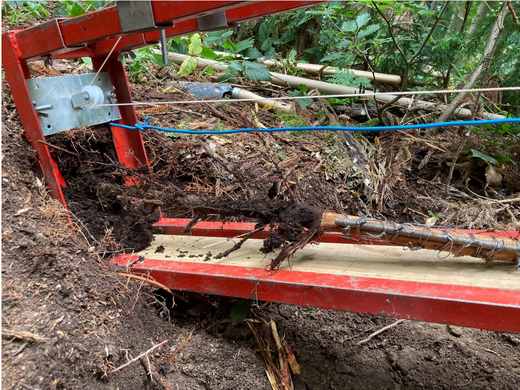
FIGURE 4.4: The Figure shows the pullout machine specially made to perform tensile tests on roots. This machine is equipped with a pulling system connected to a winch, a load cell to measure the force, a displacement sensor to measure the root displacement, and a datalogger for measuring data. In the anchoring process, the root, debarked, must be tied to a threaded bar with a ring to allow connection with sensors and the machine itself. The test begins when the root is subjected to tension force and proceeds until its complete failure.
