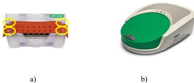
Figure 19: a) preparing the droplet generator cartridge to be placed into the droplet generator by securing a gasket over it, b) Bio-Rad droplet generator
