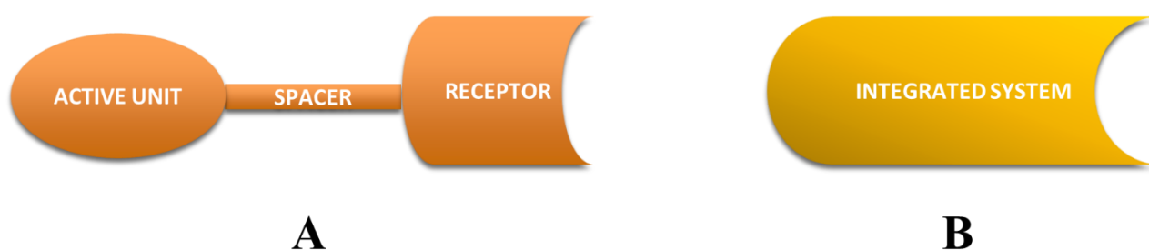
Figure 1. Schematic representation of a generic chemosensor designed following the “receptor – spacer - active unit” (A) and “integrated system” (B) approaches.
