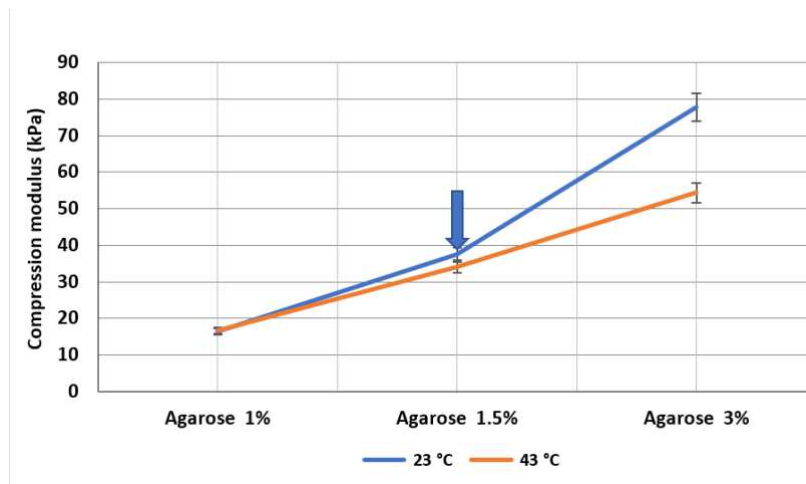
Figure 6F. Dependence of the Young's modulus of elasticity on agarose concentration.
