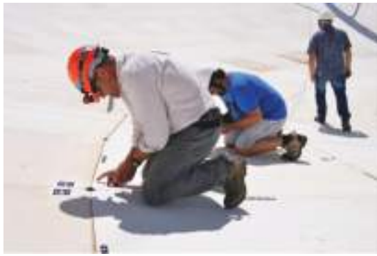
Figure 2. Setting up photogrammetric measurements at the SRT.
