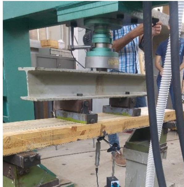
18 19 20 21 22 23 24 25 26 27 28 29 30 31 32 33 34 35 36 37 6 38 39 7 Fig. 5. Loading set-up for bending test of 60-PF CLT specimens. 40
