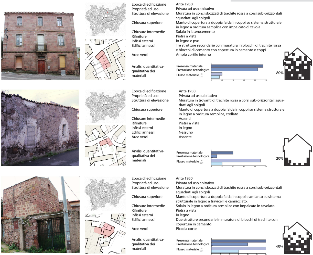
Figure 4. Filing of building: material consistency; residual performances; in and out material flow (drawings by Paloma Deidda).
